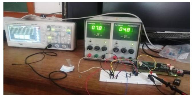
Figure 14 IGBT switching test hardware setup using DSP-C2000
