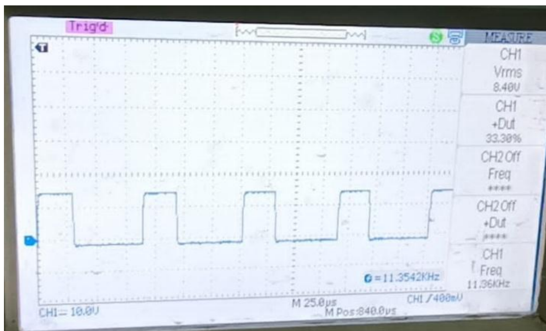
Fig-10: Pulse of MOSFET
