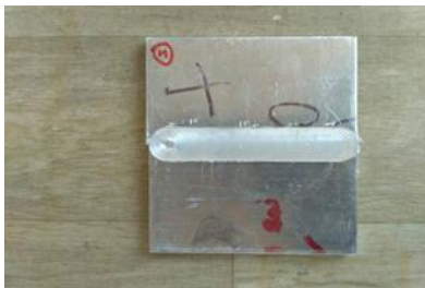
Fig.2.3. Friction Stir Welded Aluminum 6082 With 0.75mm root gap at 1400 rpm
