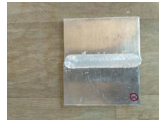
Fig.2.6. Friction Stir Welded Aluminum 6082 With 0.75mm root gap at 1800 rpm
