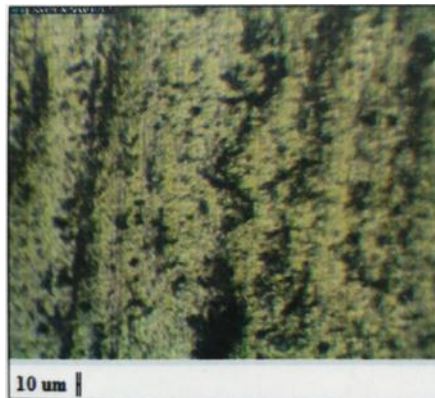
Fig.:5.11 Grain Size of 0.5 root gap specimen at 1800 rpm
