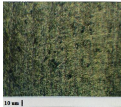
Fig.:5.5 Grain size of 0.5 root gap specimen at 1400 rpm
