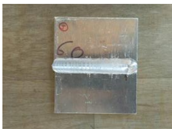
Fig.2.4. Friction Stir Welded Aluminum 6082 With 0.25mm root gap at 1800 rpm
