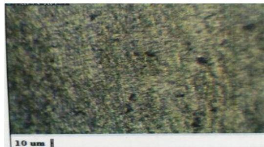
Fig.:5.13 Grain Size of 0.75 root gap specimen at 1800 rpm
