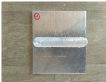
Fig.2.2. Friction Stir Welded Aluminum 6082 With 0.5mm root gap at 1400 rpm
