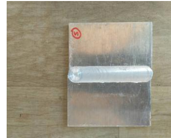
Fig.2.5. Friction Stir Welded Aluminum 6082 With 0.5mm root gap at 1800 rpm
