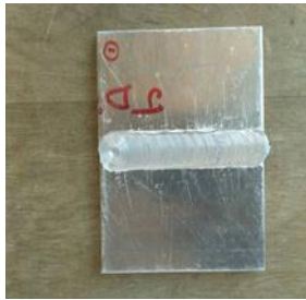
Fig 2.1. Friction Stir Welded Aluminum 6082 With 0.25mm root gap at 1400 rpm
