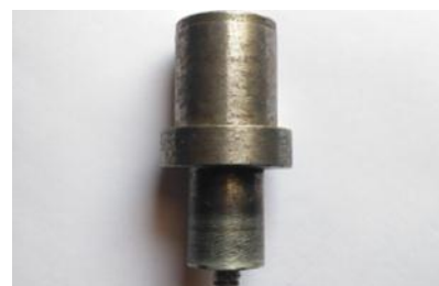
Fig 1.2. Shoulder Shaped tool used For Friction Stir Welding.
