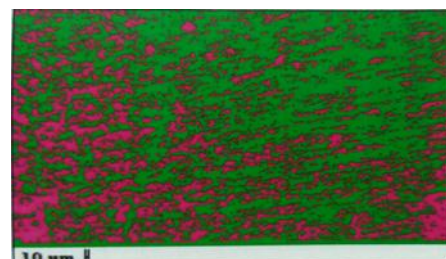
Fig.:5.8 Heat affected zone of 0.75 root gap specimen at 1400 rpm
