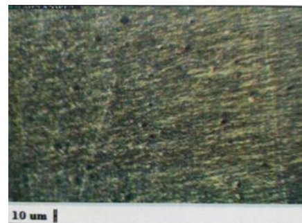
Fig.:5.7 Grain Size of 0.75 root gap specimen at 1400 rpm
