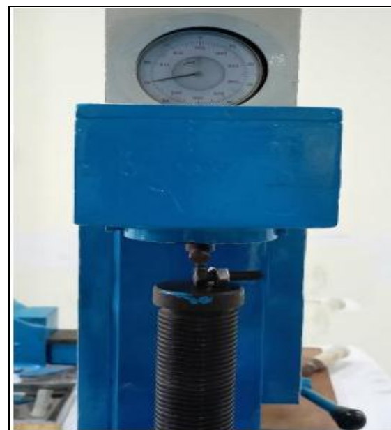
Fig -5: Rockwell hardness
