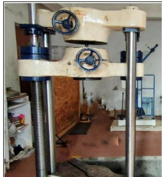
Fig -4: Universal testing machine (UTM)
