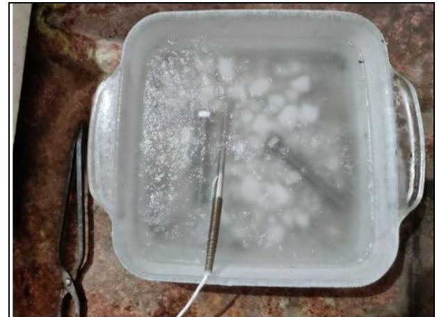
Fig -2: Bolts dipped in a mixture of Dry-ice and Acetone
