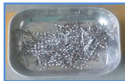
Fig-2 Crimped steel fiber
