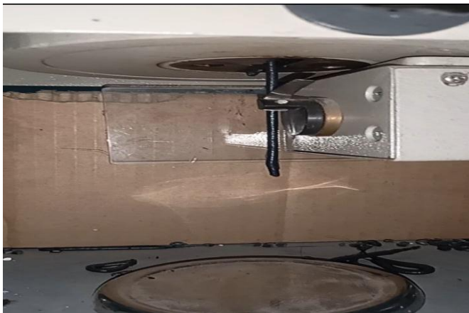
Fig 1 Strands of various granules composition produced in MFI machine.
