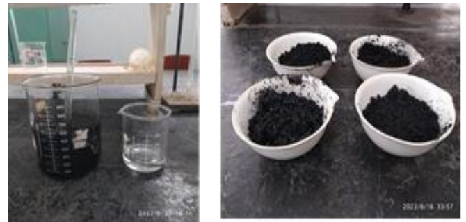
Fig. 2.3 Chemical activation of watermelon rind
