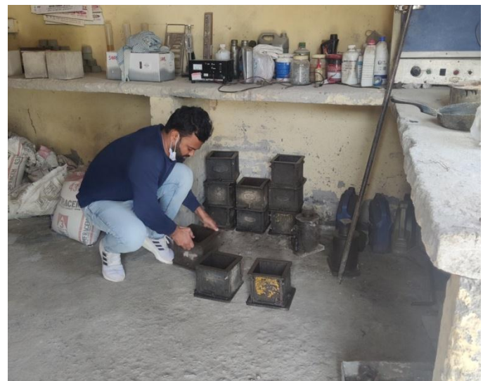
Fig. 2 Casting of cubes
