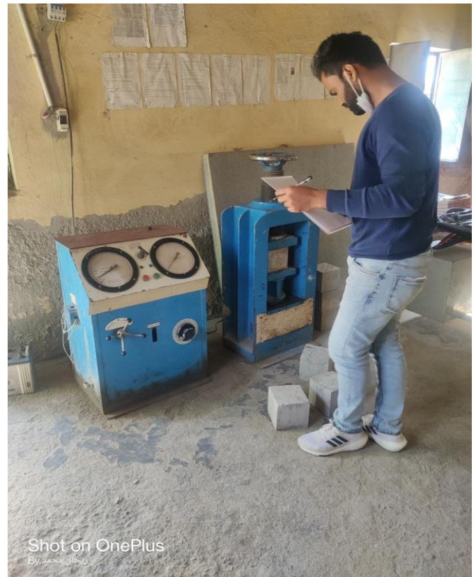
Fig. 4 Performing the compressive test on cubes in compression testing machine
