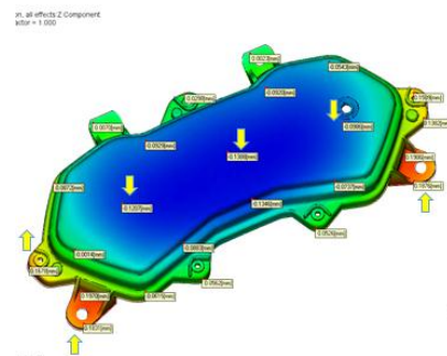
Figure 11: Z direction deflection
