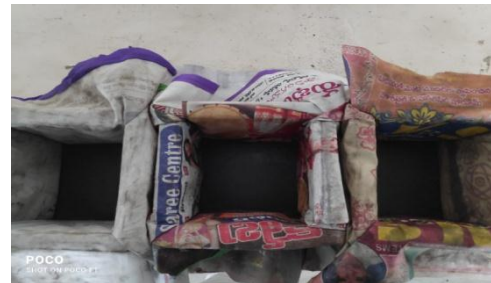
Fig.5 controlled permeable formwork
