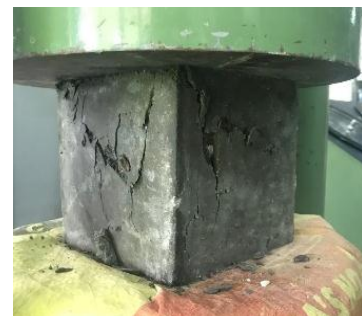
Figure 2 Compressive Strength Test of SCC Mix with GGBFS
