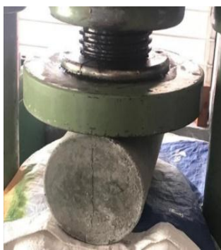
Figure 3 Split Tensile Strength Testing of LWSCC Mix with GGBFS
