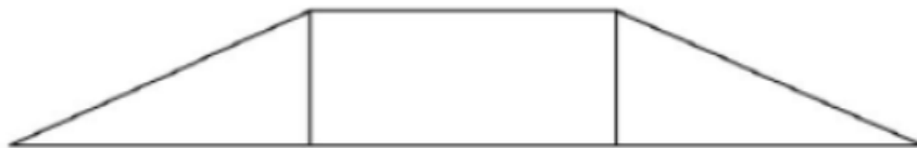
Fig 4.3: Bending moment diagram
