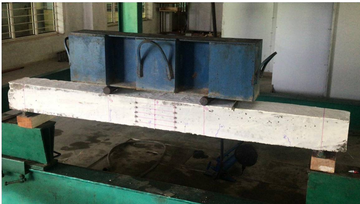
Fig 4.3.1: Testing of beams before retrofitting and initial cracks are marked
