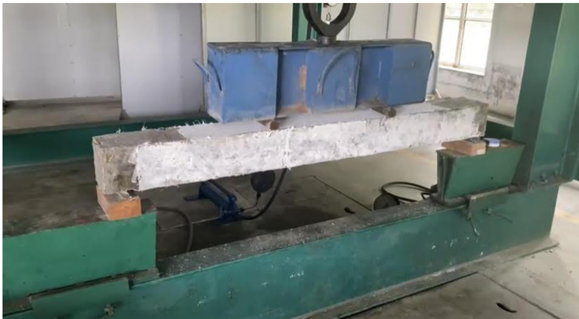
Fig 4.4.3: U wrapped collapsed beam for retrofitting
