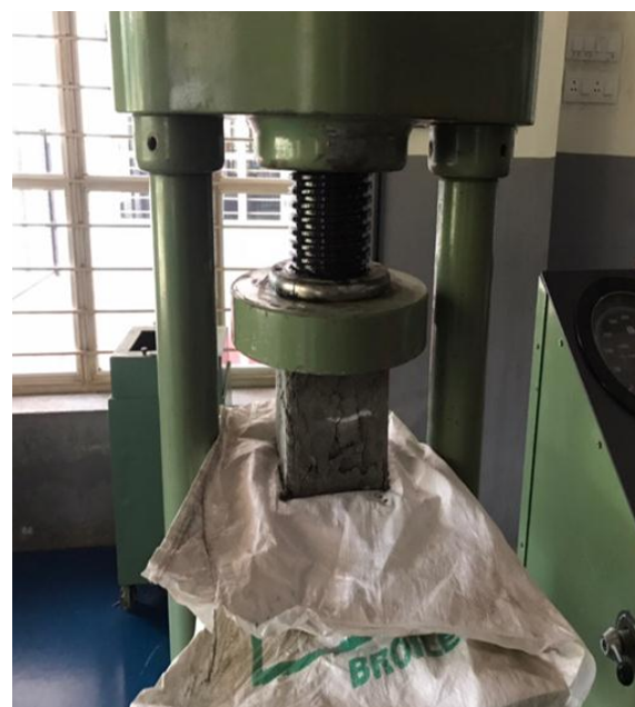
Fig 4.1.2: Compression test for cube specimen
