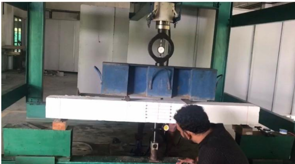
Fig 4.4: Experimental set up for beams
