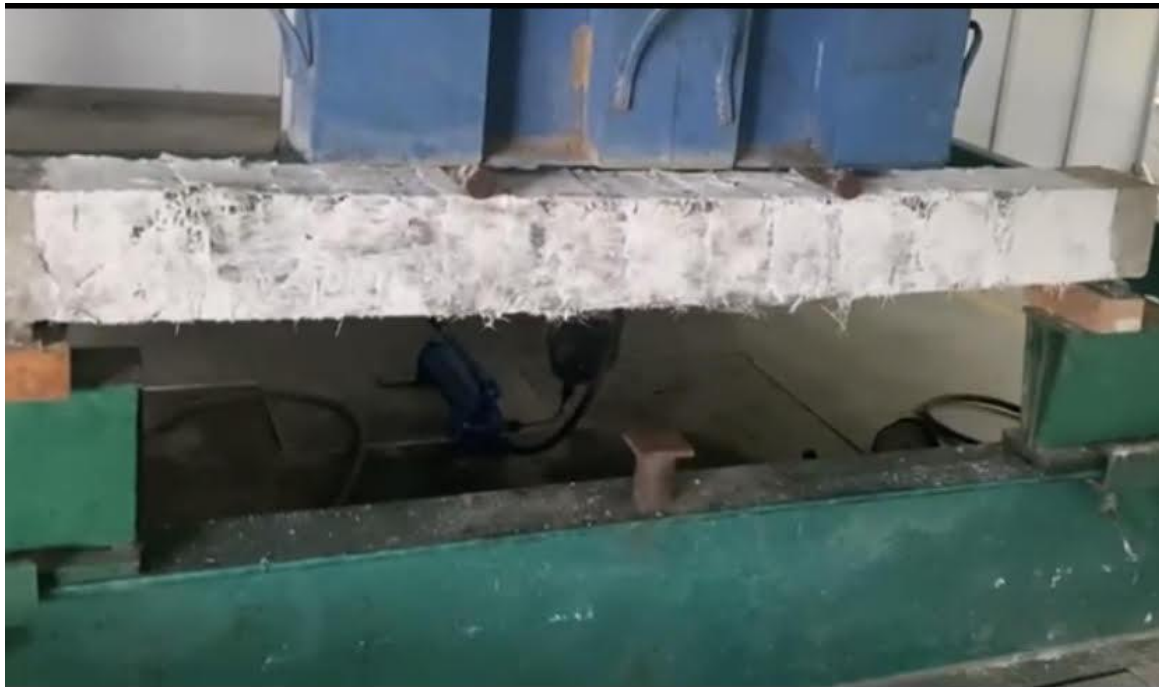
Fig 3.4: Combination of 45degree and 90 degree strip wrapping using glass fiber sheets (white cement applied)
