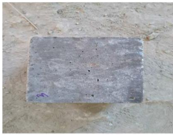
Fig 4.1.1: Unmoulded specimen for testing
