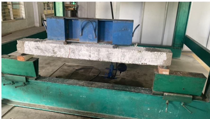
Fig 4.3.3: Testing of beams after retrofitting with wrapped glass fiber sheets
