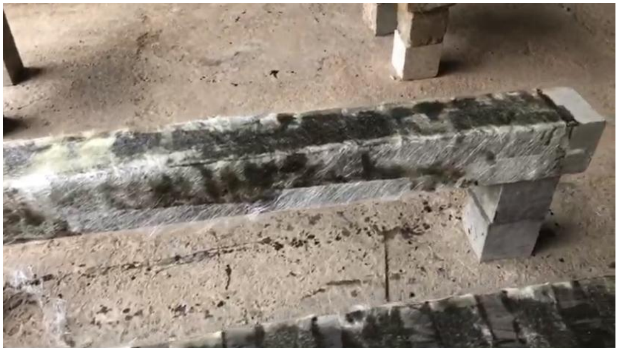
Fig 3.1: Application and fixing of glass fibre sheet and resin mortar
