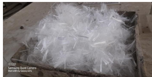
Fig. 2: polypropylene fibre (24mm)
