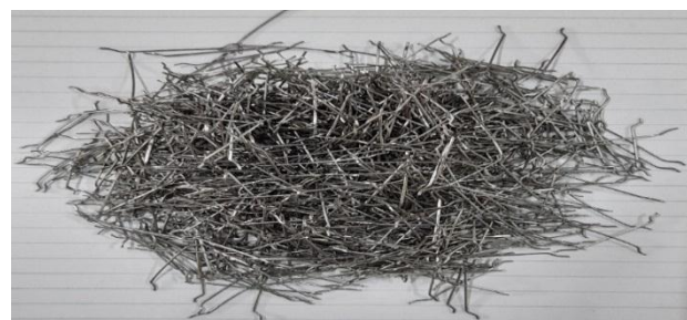
Chart - 1: End hooked steel fibre (30mm)
