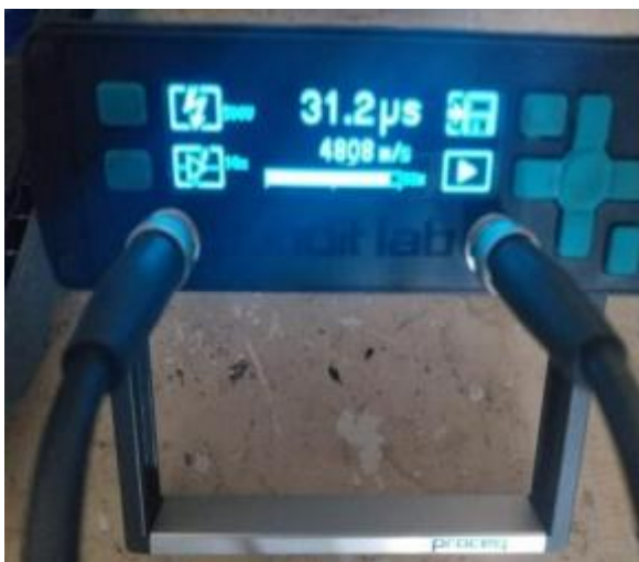
Fig 3.2 Ultrasonic pulse velocity test setup
