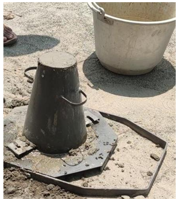
FIG-3: Slump cone test on concrete
