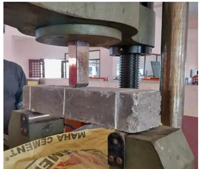
Fig-9: Flexural strength test on concrete
