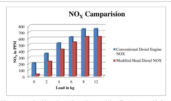
As compared  $NO_X$  emission is reduced due to the complete combustion and also sufficient air is passed for burning which also act as cooling agent that reduces the internal temperature of the combustion chamber.
