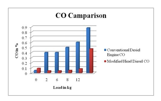
As compared CO emission is reduced significantly due to the complete combustion occurring inside the combustion chamber.
