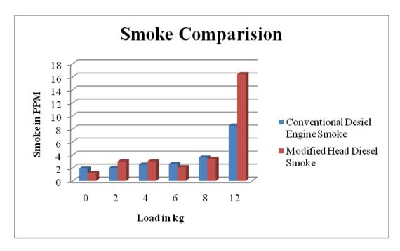
Due to combustion of rich fuel in the modified engine head smoke is slightly increased with load.
