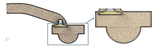
The fundamental benefit of polyhedral meshes is that each cell has a high number of neighbors, allowing for precise gradient approximation. Furthermore, polyhedrons are less prone to stretching than tetrahedrons, resulting in greater mesh consistency and numerical stability of the system. Furthermore, numerical diffusion is reduced due to mass interchange across several faces. As a result, the answer is more exact with a somewhat lower count.
