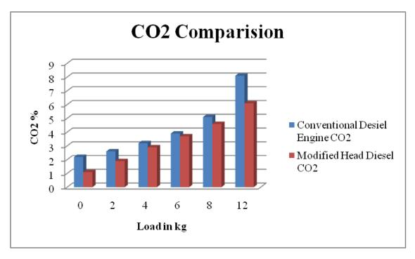
As compared CO<sub>2</sub> emission is reduced slightly due to the complete combustion occurring inside the combustion chamber.
