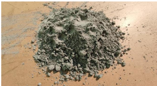
Fig -1 WASHED BOTTOM ASH
