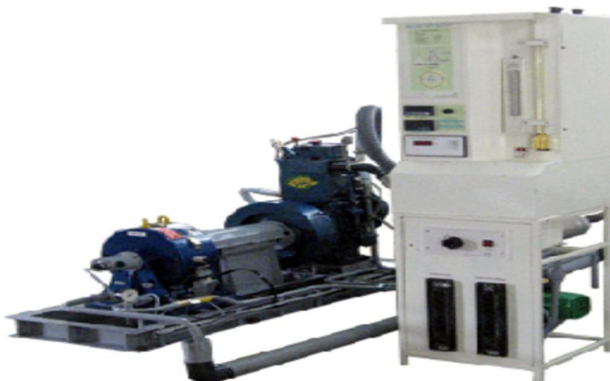
Fig-6: Computerised diesel engine test rig
