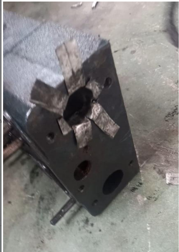
Fig-5: Swirl enhancer inserted in a cylinder head
