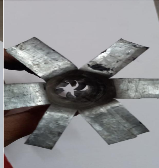
Fig-3: Top view of the swirl enhancer
