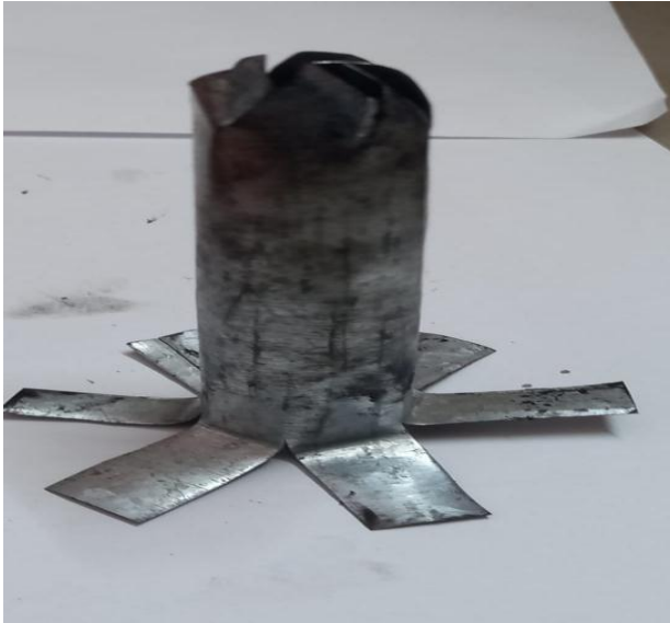
Fig-2: Side view of the swirl enhancer
