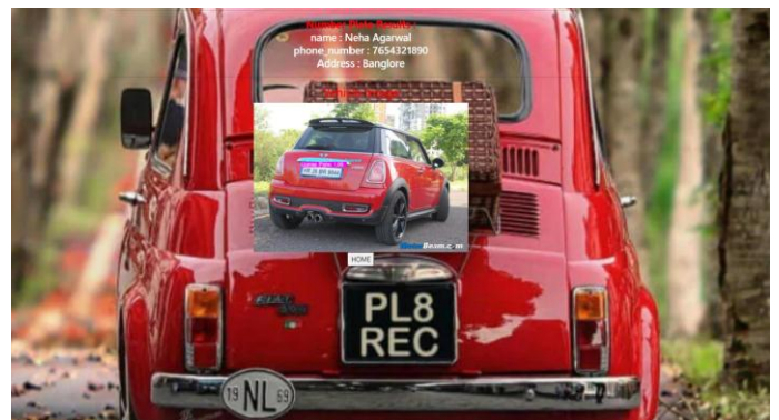
Fig 5.7 Snapshot 2 of vehicle ownership details extracted from database after number plate detection
