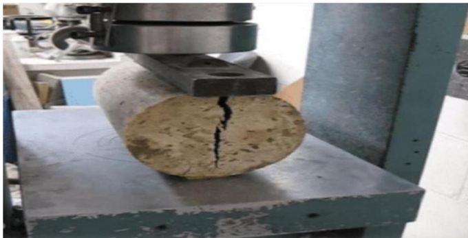
Fig-4: Split tensile strength test
