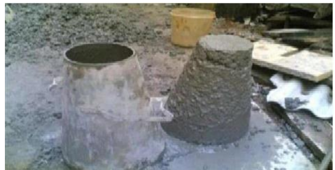
Fig-2: Slump cone test
