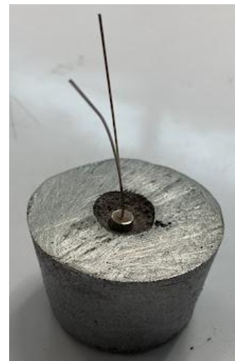
Figure 3. Cartridge heater and aluminum sheath
