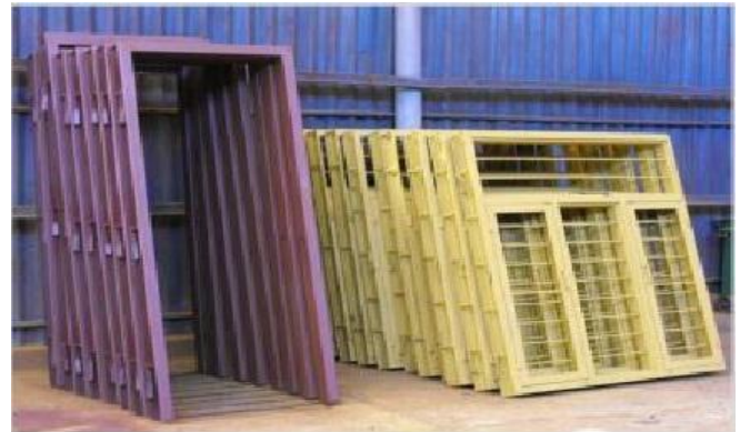
Fig. No. 8 Prefabricated windows and door frames
