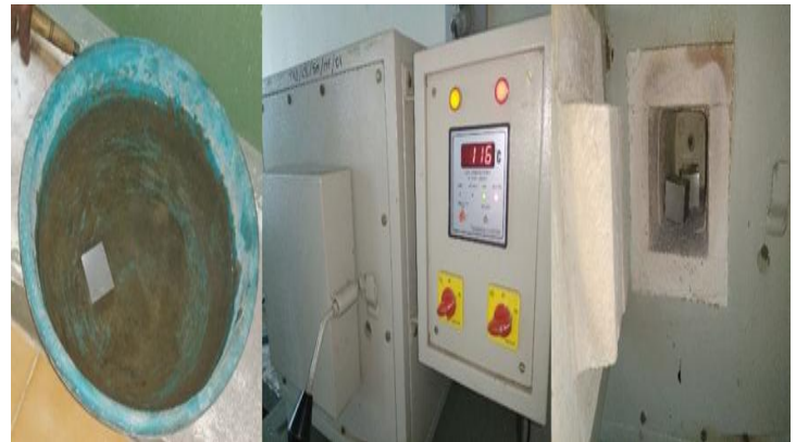
Fig. 2 – Heat treatment of Al6061 cast specimen with the mono and multi heat treatment methods.
