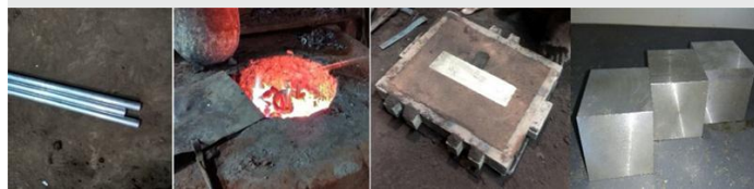
Fig. 1 – Preparation of specimen by stir casting of Al 6061.
