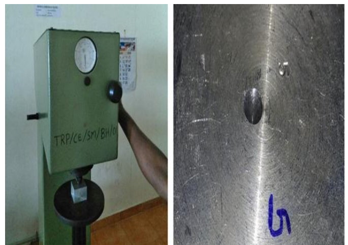
Fig. 4 – Hardness testing and its impression on heat treated hot pressed Al6061 casted specimen.
