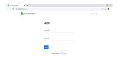
Firstly, the client/user needs to enter the login Id and secret key which are unique provided by the organization. When that coordinates with the data set, the next phase is to create the OTP on the enlisted phone number. If the user is failed to provide the OTP, further access to the system is denied. If the OTP is accurate, the user is directed to the next phase.
