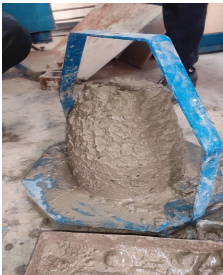
Fig -4 Slump test
