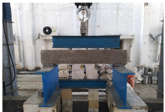
Fig - 3: Test Setup of Beam in Loading Frame for Deflection Behaviour
