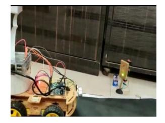
• **Lane Detection:** A trained Convolutional Neural Network model is used to predict the next move of the car. If the road is moving towards the left, the prediction given by CNN will be a left turn. During a left turn, the Model sees whitespace of the floor on the right and black chart paper on the left, which triggers a Left turn prediction.
