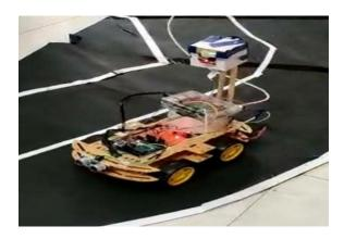
The picture depicts the hardware prototype of our selfdriving car model made using CNN and IOT devices. The black chart paper here acts as an artificial environment on which the prototype will work abiding by rules that we have stated.
