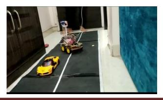
• **Traffic Signals & Road Sign Detection:** In order to detect the signals wehave a pre-trained cascade classifier model in OpenCV. A cascading classifier detects a frame as positive or negative so each classifier will check each framefor positive samples, if the sample is not found the sliding window moves to the next frame. The next frame is checked again for a particular classifier. Thisgoes on till the entire frame of the video is covered.
