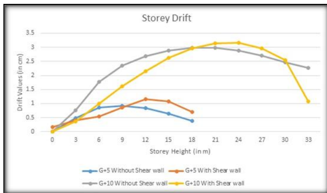
Chart -2: Graph for comparing the storey drift values between Mid-rise and High-rise building with and without shear wall
