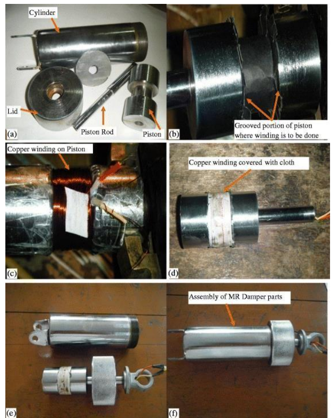
Fig-3 Making of MR Suspension
