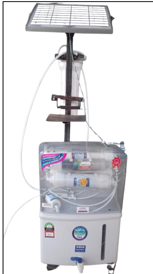
Fig: Solar based Water Purifier
