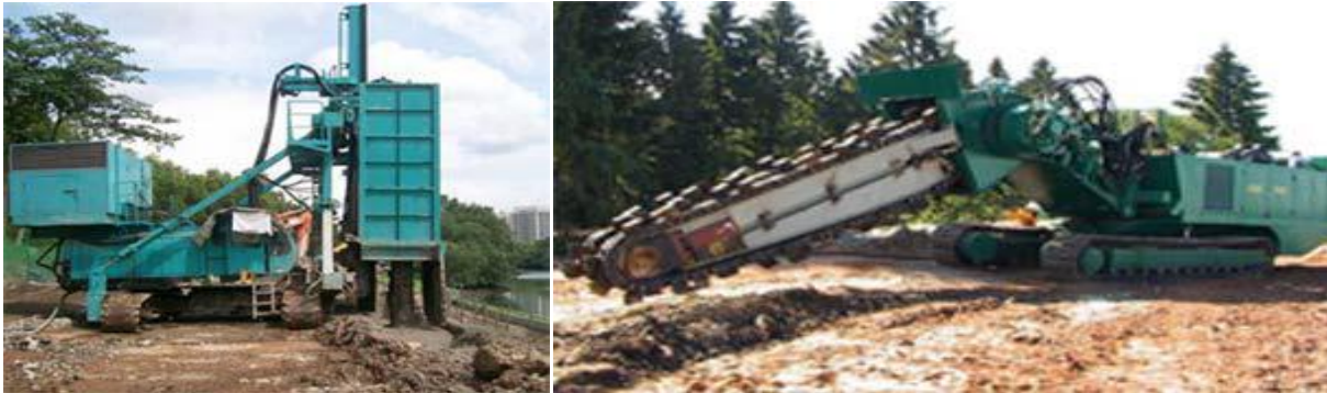
Figure 2: The FMI and TRD–Trenching machine for construction of deep walls (Massarsch and Topolnicki, 2005; Hayward Baker Inc.)
