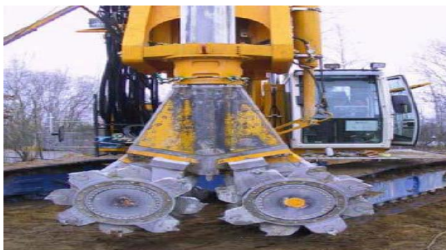
Figure 4: Bauer cutter soil mixing (Fiorotto et al, 2005)
