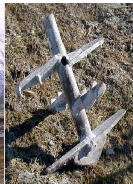
Figure 5: Nordic modified dry mixing tool (Larsson, 2005)
