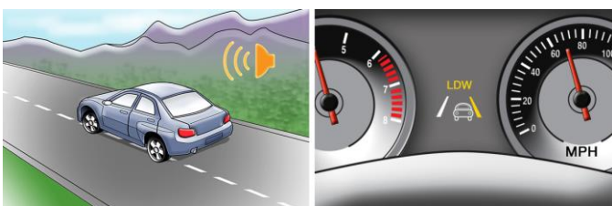
Lane departure warnings[4]
