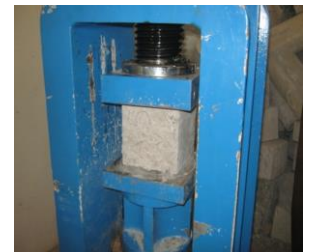
Fig. 6: Testing of cube.
