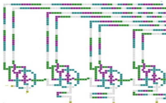
Fig 3(c): Proposed design of QCA cells in 4-bit adder
