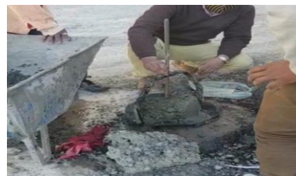
Fig - 1: Slump test
