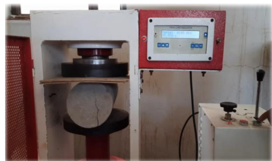
Fig - 3: Split tensile test
