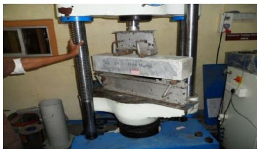
Fig - 4: Flexural strength test
