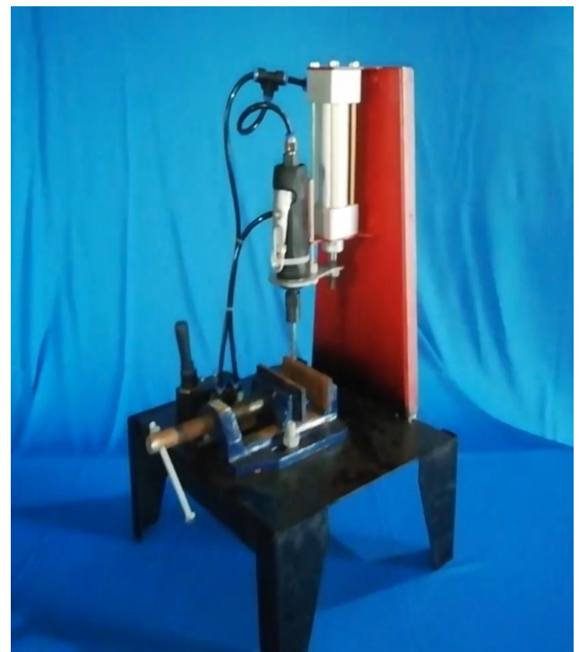
Fig -6: Pneumatic auto feed drilling machine – Photographs
