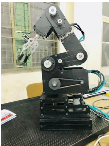
Figure 1: Mechanical design of 6-DoF robotic manipulator, including six servo-DC motors, belt-pulley mechanism to enhance torque, control unit, and functional gripper
