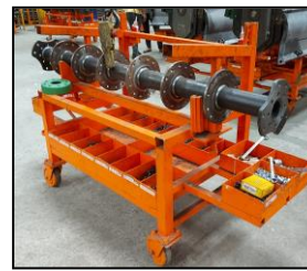
Fig-2: Assembly Trolley with rotor shaft
