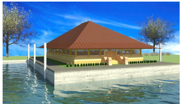
Fig -8: A conceptual model of an amphibious house during floatation condition integrated with the vernacular architectural style.
