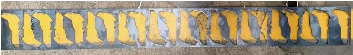
Fig -13: Arrangement of punching of the levers in the implemented process.
