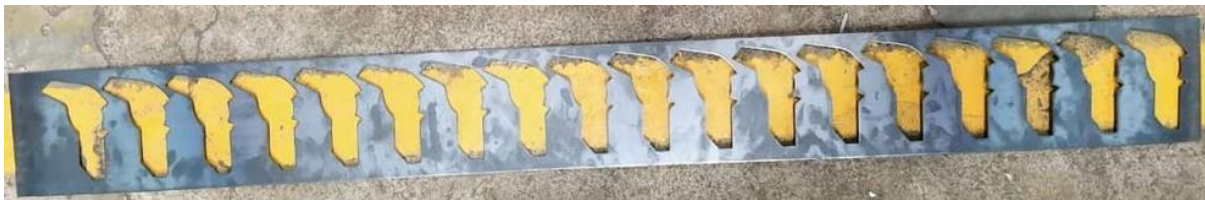
Fig -10: Arrangement of punching of the levers in the initial process.
