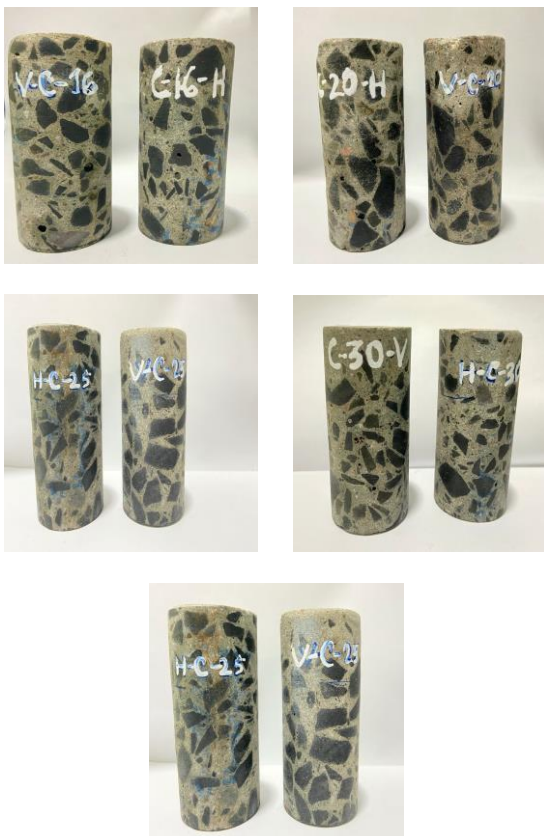
Figure 4: Core samples at various direction of drilling i.e. H-Horizontal direction of drilling (Perpendicular to the direction of pouring) & V-Vertical direction of drilling (Parallel to the direction of pouring) for different grade of concrete.
