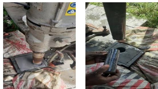
Figure 2: Drilling of Core sampling from cube samples.
