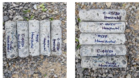
Figure 3: Core specimens collected from cube samples.
