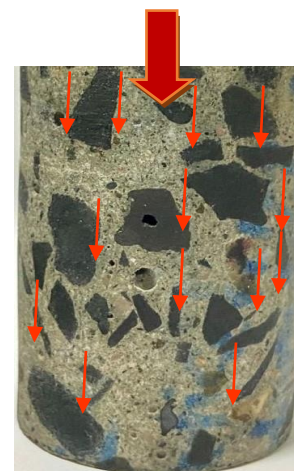
Figure 5: Loading direction parallel to weakest ITZ between aggregate & paste structure when direction of drilling is Perpendicular to the direction of pouring.
