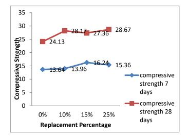
As shown in the graph: (7 days strength), when sand is partially replaced 10% by CERAMIC WASTE, compressive strength is increased by 19.9 %. 28 days strength in graph: show an increment of 26.85% of strength of 25% replacement of CERAMIC WASTE as compared with conventional concrete.
