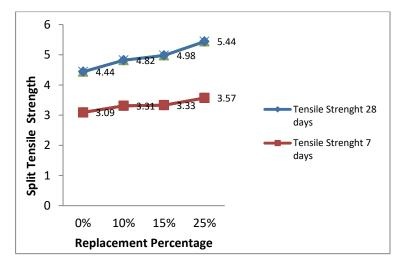
As shown in the graph: 9 (7 days strength), when sand is partially replaced 10% by CERAMIC WASTE i.e., Split Tensile strength is increased by 38%. Afterwards when % of CERAMIC WASTE is increased the strength starts decreasing
