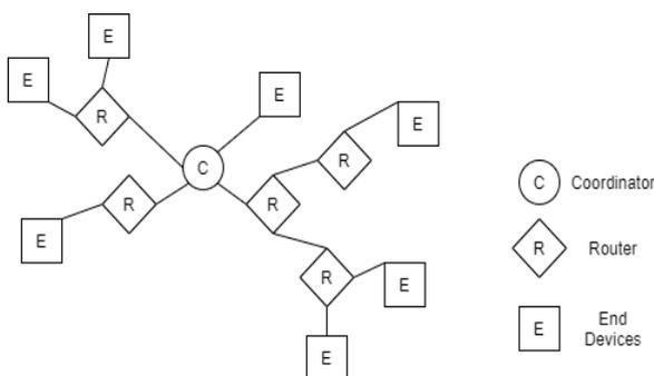
Figure 1: Mesh topology of ZigBee Devices
