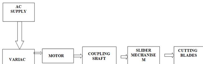
Figure 2.2 Block Diagram
