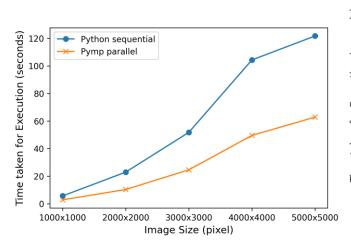
Chart - 2: Graph of execution time for Otsu segmentation using Python
