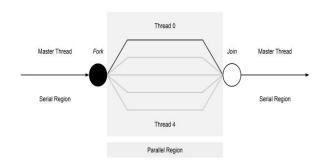
Fig – 1: OpenMP master-thread architecture
