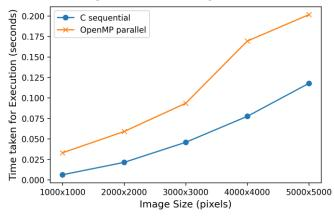
Chart – 1: Graph of execution time for Otsu segmentation using C
