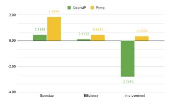
Chart – 7: Mean performance metric of all image sizes for Otsu segmentation
