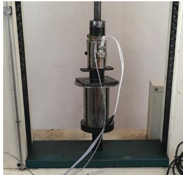
Fig -2: Pressed cylinder equipped with band heater
