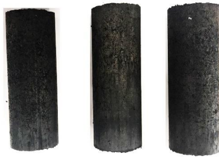
Fig -3: Briquettes from leftover charcoal
