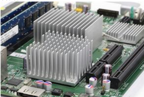
Fig 1.1 Heat Sinks placed on a motherboard.
