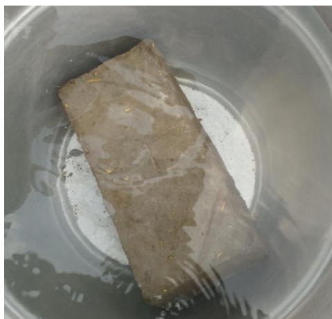
Fig -5: Water Absorption Test on Brick
