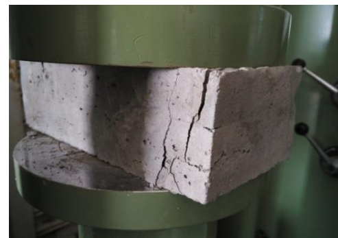
Fig -4: Compressive Strength Test on Brick
