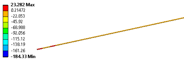
Fig 8.3: Minimum principal stress of hallow shaft.
