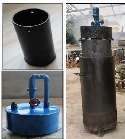
Fig -2: Pictorial view of existing open top gasifier and developed steam activation unit
